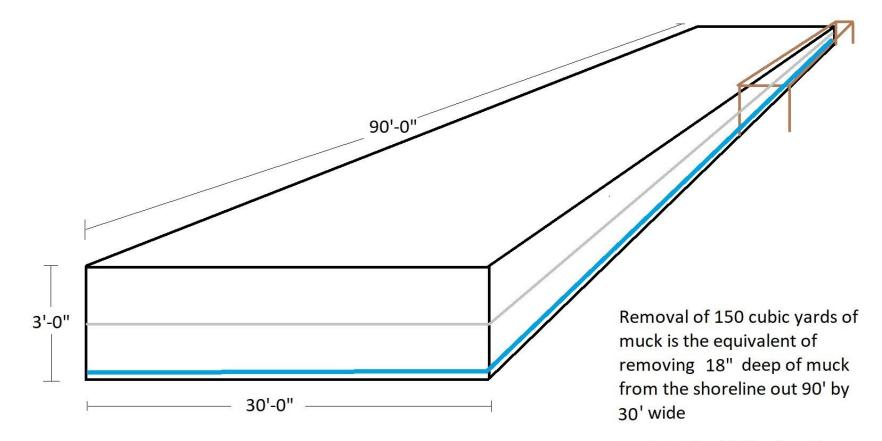
or removing 3'-0" of muck from a 30' wide path from shore out 45'
